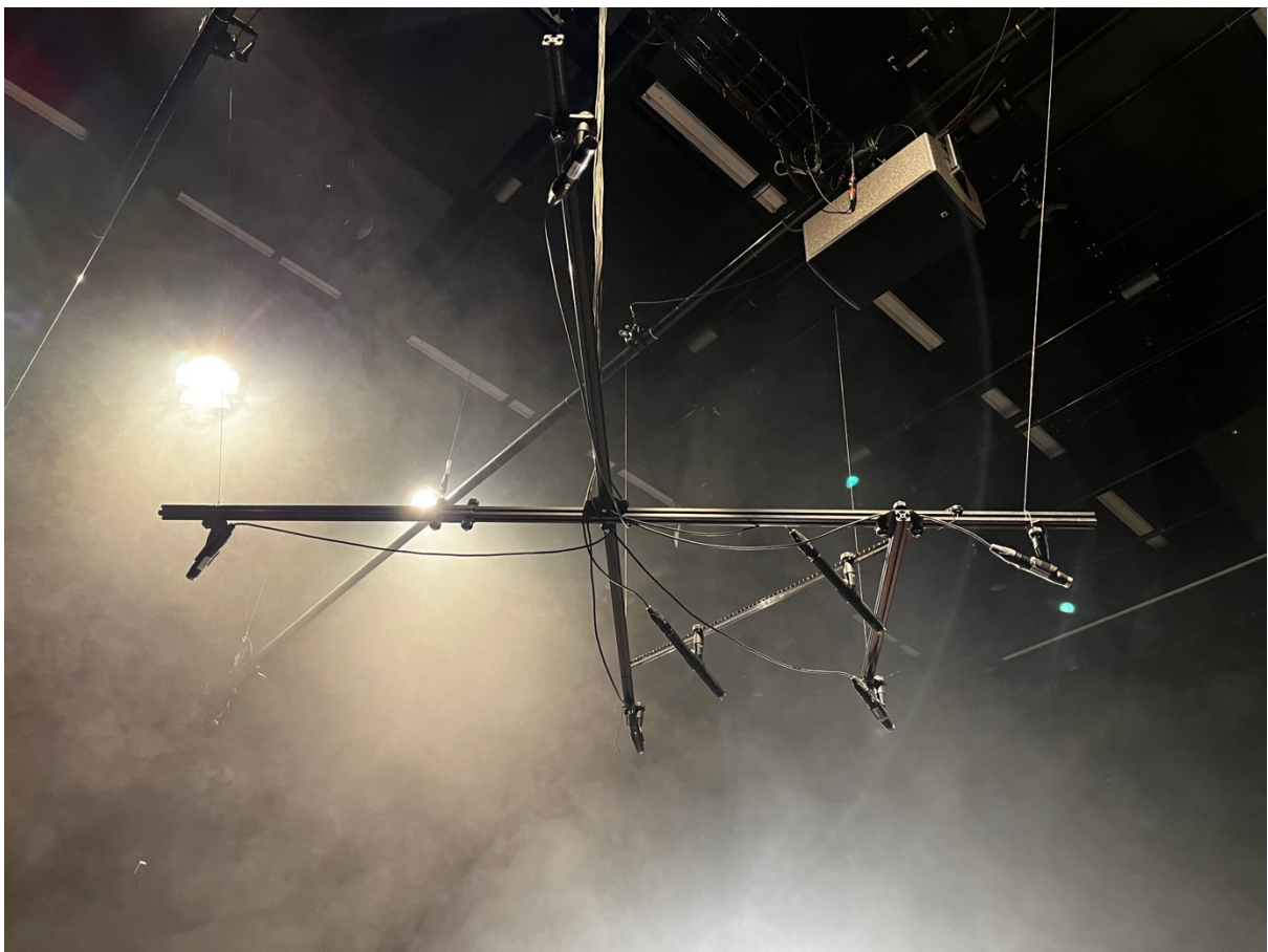
Figure 19 View of the modified 2L-Cube with the additional AB array. One of the truss-mounted top layer microphones can be seen (own photograph).
